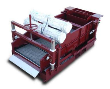
The SCM PrimaG shaker is a Linear Motion shale shaker which produces 7.3 g's of vibrational force. The PrimaG 4P Linear Motion shale Shaker has been designed with an impressive 30  $\rm ft^2$  of screening area while maintaining a small equipment footprint. The large screen area of 30  $\rm ft^2$ , 7.3 g's of force and linear motion results in excellent solids conveyance and outstanding performance.
